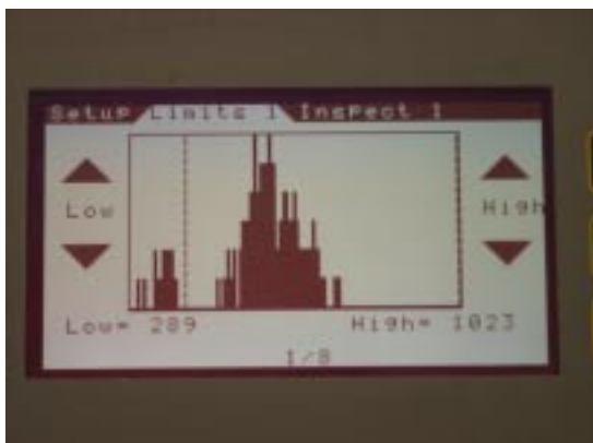
Discriminate between sealed and leaking containers through onscreen histograms.
